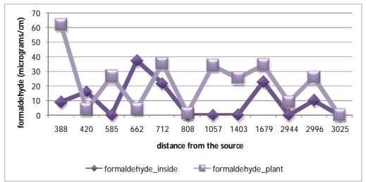
Figure 2. Distribution by distance of the formaldehyde concentrations measured simultaneously inside the selected houses in the residential area and at the plant.
